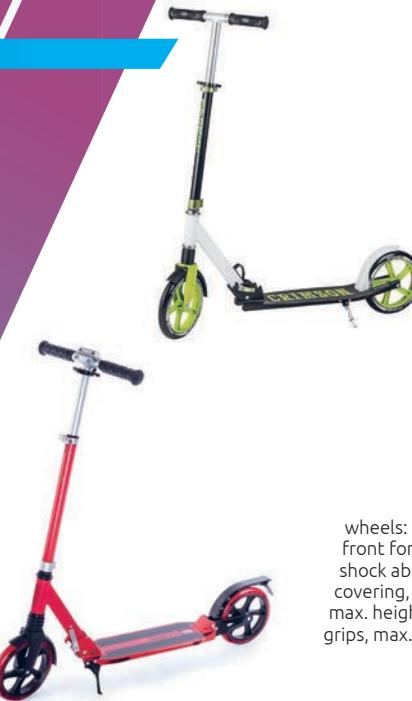
wheels: 230 mm PU, bearings: ABEC7 ZZ, material: 100% aluminum, antisliding tread, max handlebar height: 109 cm, foldable, rear friction brake, soft hand grips, deck: 58x15 cm, weight: 4,85 kg, max user weight: 100 kg, standard EN 14619, packing: 2 pcs/carton
