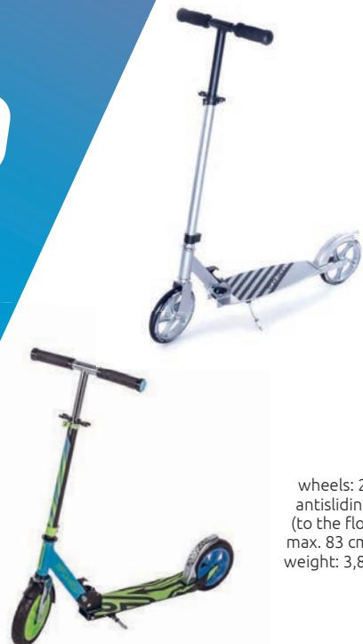
wheels: 200 mm, pneumatic, rubber, bearings: ABEC7 2RS, material: 50 % aluminium, antisliding tread, deck: 54x11,5 cm, max. height of the handlebars: 89,5 cm (to the floor), min. height: 77 cm (to the floor), counted from the platform: max. 83 cm, min. 71 cm, foldable, rear friction brake, soft hand grips, kickstand weight: 3,8 kg, max user weight: 100 kg, standard EN 14619, packing: 4 pcs/carton
