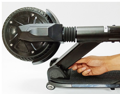
Unfolding Press the button by hand
